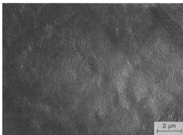
Figure 7 Banded spherulite of sol fraction, T_c = 92^\circ\text{C}
